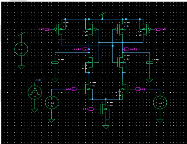
Fig2.1. Schematic diagram of single-tail dynamic comparator.
