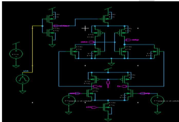
Fig3.1. Schematic diagram of Conventional Double-tail dynamic comparator.
