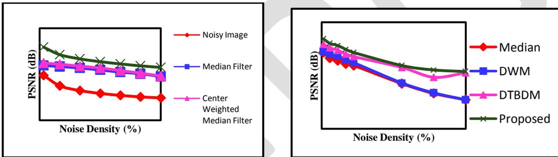
Fig. 5. Comparison graph of various denoising method
