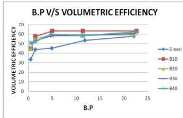
In the above graph Brake power is taken in x-axis and Volumetric Efficiency should be taken in y-axis. The volumetric efficiency of the blends has been compared with diesel fuel at various loads and it is shown in figure. It is observed that the Volumetric Efficiency for B40 blend was considering Higher over entire load range.
