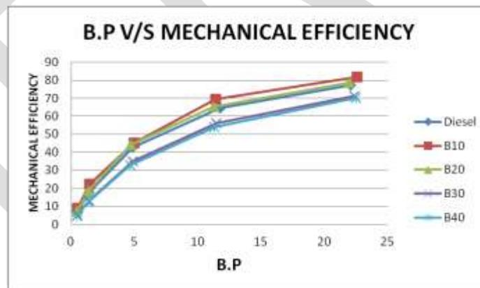
In the above graph Brake power is taken in x-axis and Mechanical Efficiency should be taken in y-axis. The Mechanical efficiency of the blends has been compared with diesel fuel at various loads and it is shown in figure. It is observed that the Mechanical Efficiency for B20 blend was considering Higher over entire load range
