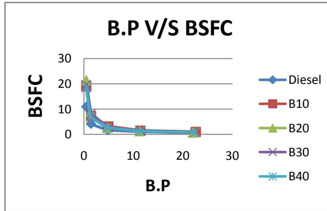
In the above graph Brake power is taken in x-axis and is taken BSFC in y-axis. The BSFC of the blends has been compared with diesel fuel at various loads and it is shown in figure. It is observed that the BSFC is less for the B20 Over the entire range of load.
