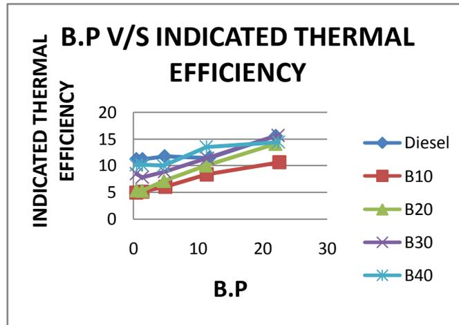
In the above graph Brake power is taken in x-axis and Indicated Thermal Efficiency should be taken in y-axis. The Indicated Thermal efficiency of the blends has been compared with diesel fuel at various loads and it is shown in figure. It is observed that the Indicated Thermal Efficiency for B40 blend was considering higher for first four loads remaining B30 is higher over the other blends operation over entire load range.
