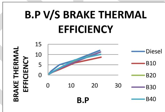
In the above graph Brake power is taken in x-axis and Brake Thermal Efficiency should be taken in y-axis. The Brake Thermal efficiency of the blends has been compared with diesel fuel at various loads and it is shown in figure. It is observed that the Brake Thermal Efficiency for B40 blend was considering higher for first three loads remaining B20 is higher over the other blends operation over entire load range.
