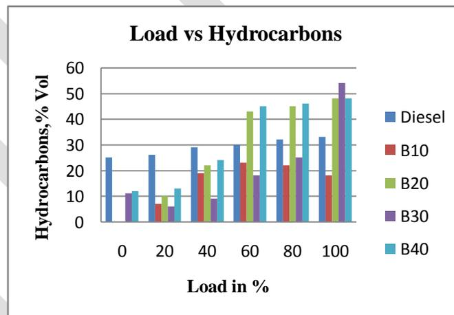
The variation of hydrocarbons with load for tested fuels is depicted in Fig. 8.. From the results, it can be noticed that the concentration of hydrocarbon of cashew nut oil and cottonseed oil blends –Diesel fuel blends is less than Diesel fuel. With increase in power output, the HC emission gradually increases for cashew nut oil and cottonseed oil blends –Diesel fuel blends.
