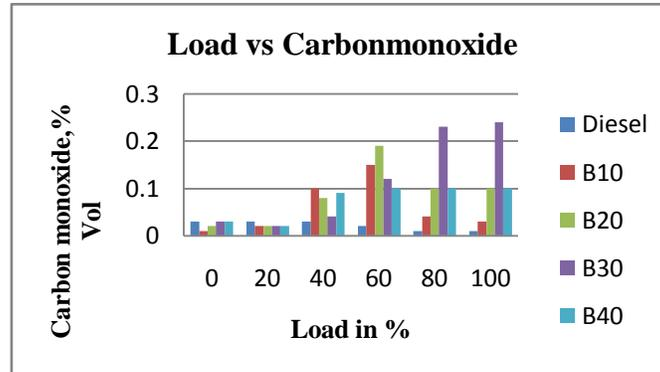
From Fig. 7, the variation of carbon monoxide with load can be observed for all the cashew nut oil and cottonseed oil blends –Diesel fuel blends. The results show that CO emission of cashew nut oil and cottonseed oil blends is lower than Diesel fuel. With increase in power output, the CO emission gradually reduces for cashew nut oil and cottonseed oil blends –Diesel fuel blends and the difference in the values for CO emission with Diesel fuel reduces significantly
