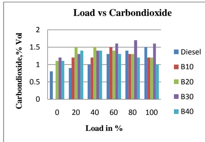
As shown in fig.9, it can be observed that the variation of carbon dioxide emission with load for Diesel Fuel and cashew nut oil and cottonseed oil blends –Diesel fuel blends. From the results, it is observed that the amount of CO<sub>2</sub> produced while using cashew nut oil and cottonseed oil blends –Diesel fuel blends is lower than Diesel fuel at all loads except full load. This may be due to late burning of fuel leading to incomplete oxidation of CO.
