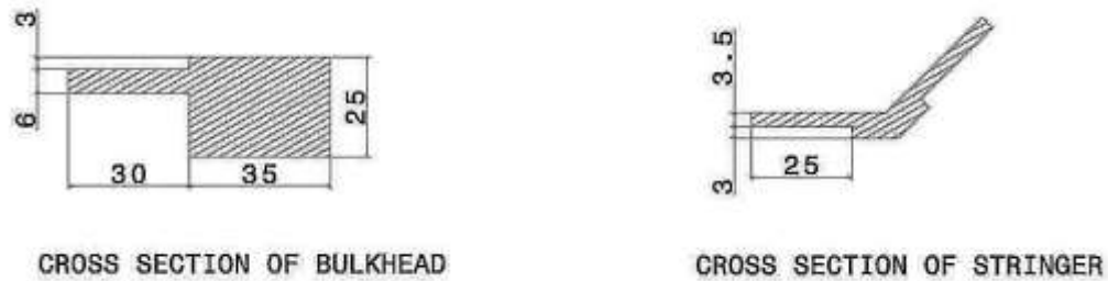
Figure 3: Geometrical configurations of bulkhead and stringer
