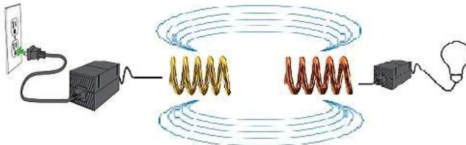
Figure 7 Energy Build Up Process in the Device Resonator due to the Source Resonator
