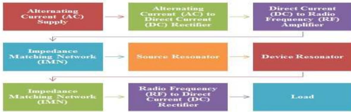
Figure 3 Block Diagram of WPT using Magnetic Resonance
