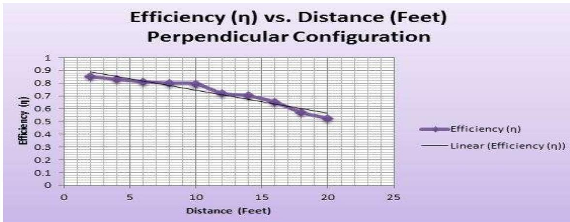
Figure 12 Efficiency vs. Distance Chart for Perpendicular Configuration
